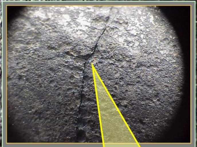
Note axial crack propagation from circ. crack
