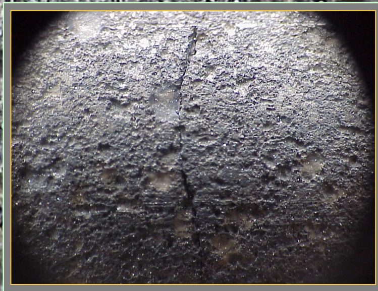
Single crack pit initiation site
