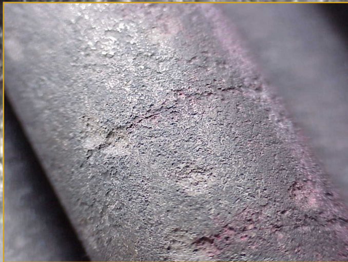
Note pitting attack along crack formation
