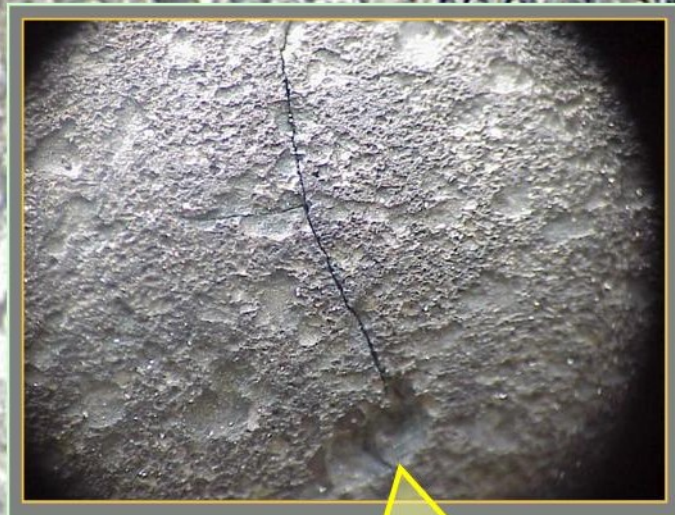
Single crack pit initiation site
