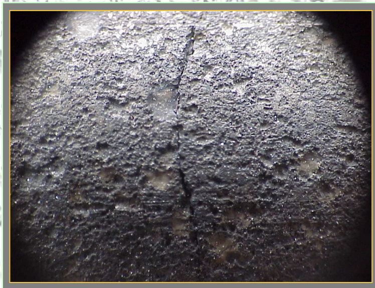
Single crack pit initiation site
