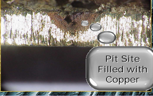
Copper Lay-out in Pit Site, Defect Depth 60%
