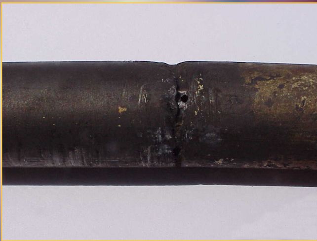
Removed tube sample: Note failure in tube
