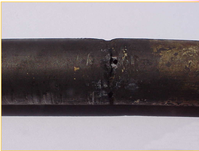
Removed tube sample: Note failure in tube
