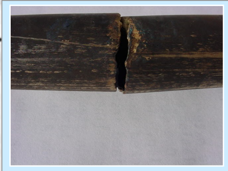
Sections from the Cracked Tubes
