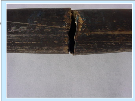
Sections from the Cracked Tubes
