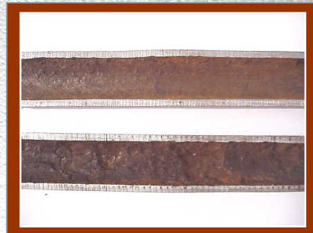
Tube Section Prior to Sandblasting
